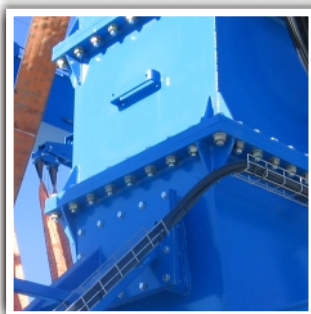
BOLTED STRUCTURE FOR EASY ASSEMBLY
